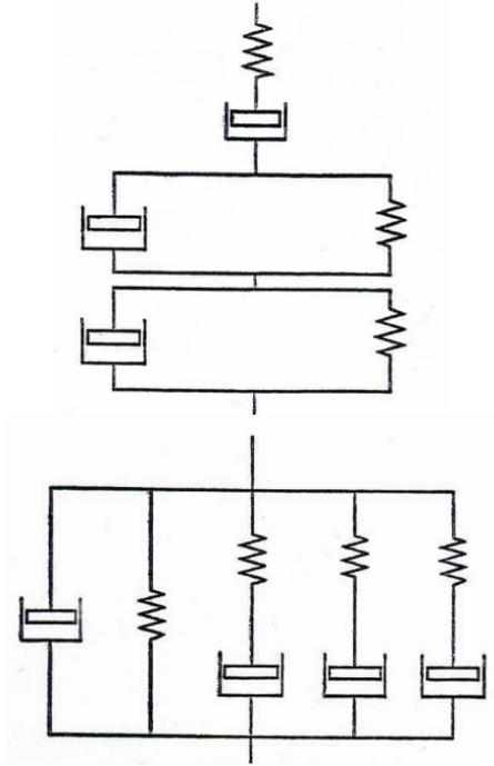
Fig. 2.4 The mechanical representations of the compound Voigt model (top) and compound Maxwell model (bottom).
